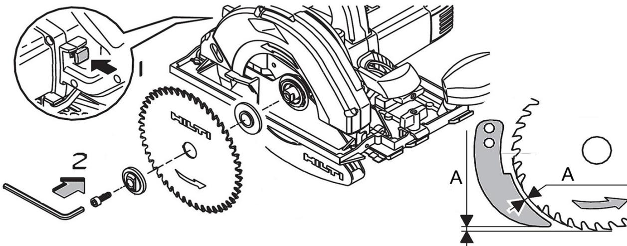
1. Rest the power tool on the ribs provided.
