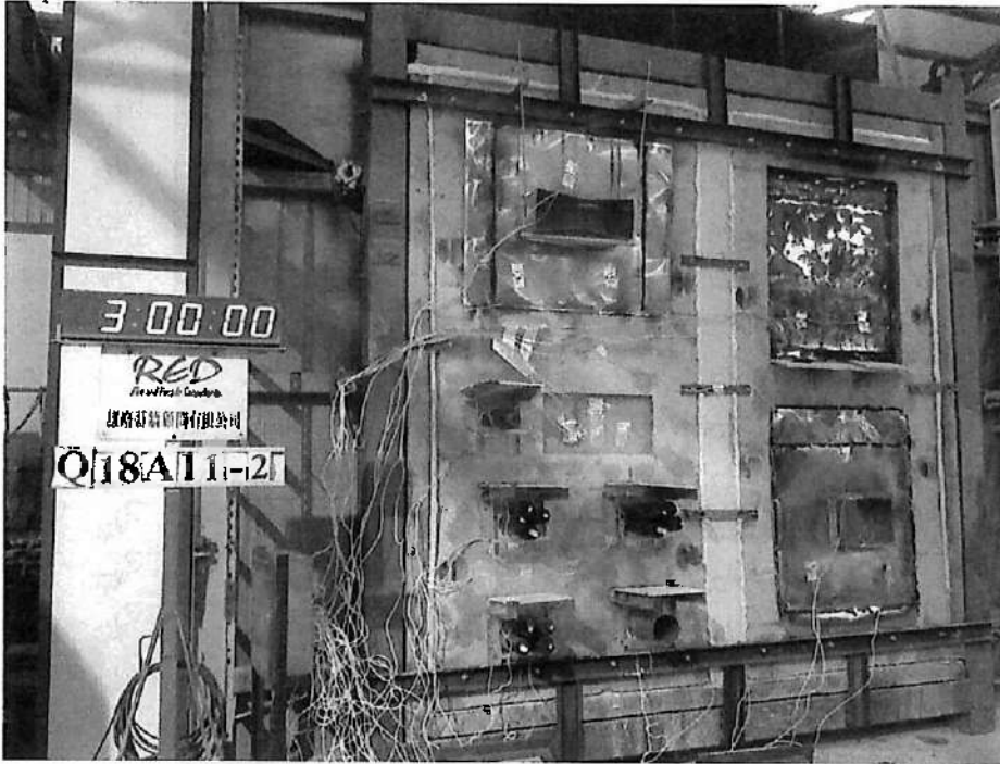
Photo 5: The unexposed face of the specimens after a heating period of 180 minutes.
