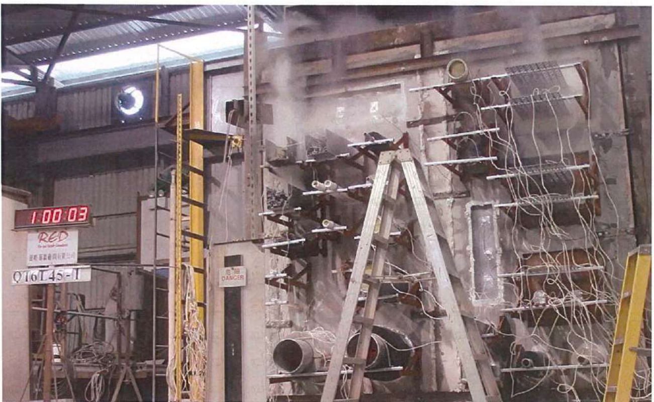
Photo 3: The unexposed face of the specimens after a heating period of 60 minutes.
