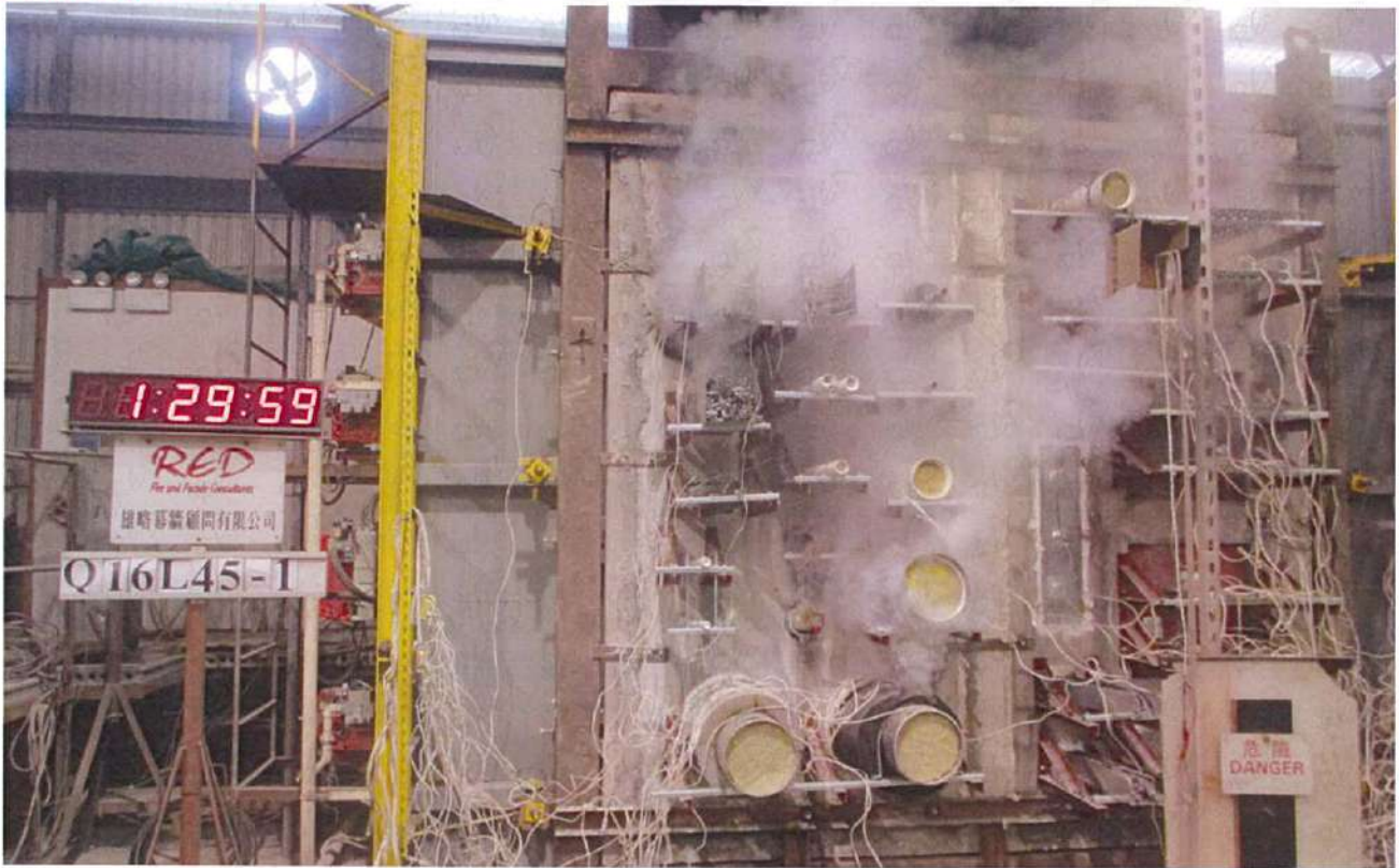
Photo 4: The unexposed face of the specimens after a heating period of 89 minutes.
