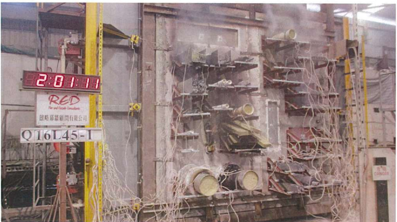
Photo 5: The unexposed face of the specimens after the test.
