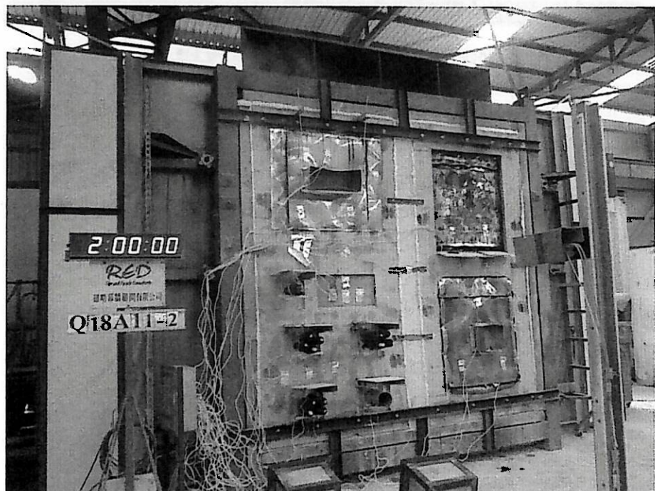
Photo 4: The unexposed face of the specimens after a heating period of 120 minutes.
