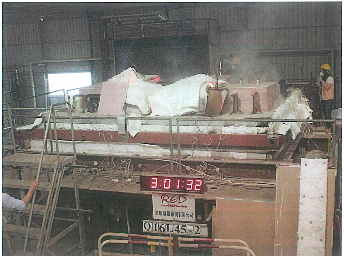
Photo 5: The unexposed face of the specimens after a heating period of 181 minutes.
