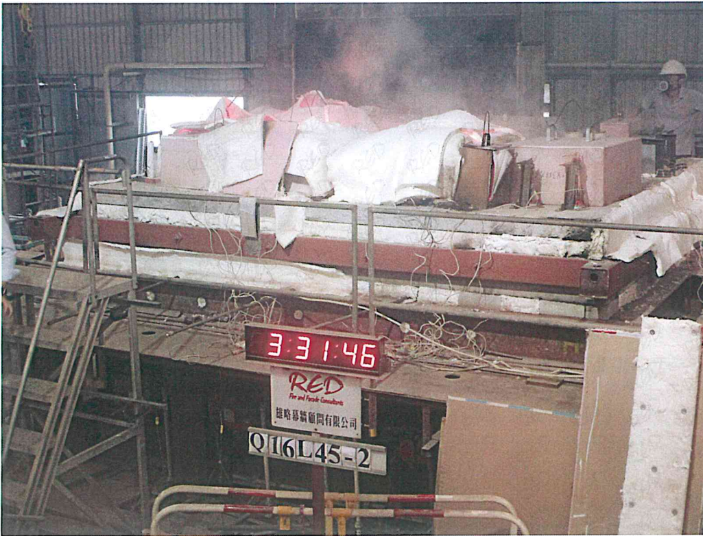
Photo 6: The unexposed face of the specimens after a heating period of 211 minutes.
