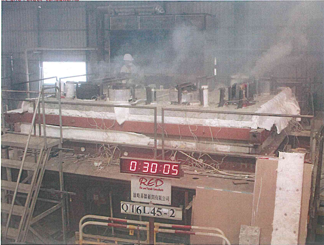
Photo 2: The unexposed face of the specimens after a heating period of 30 minutes.
