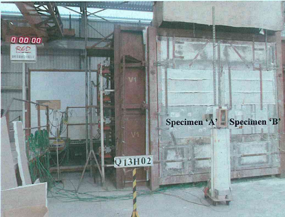
Photo 5 - The unexposed surfaces of the specimens before the test.
