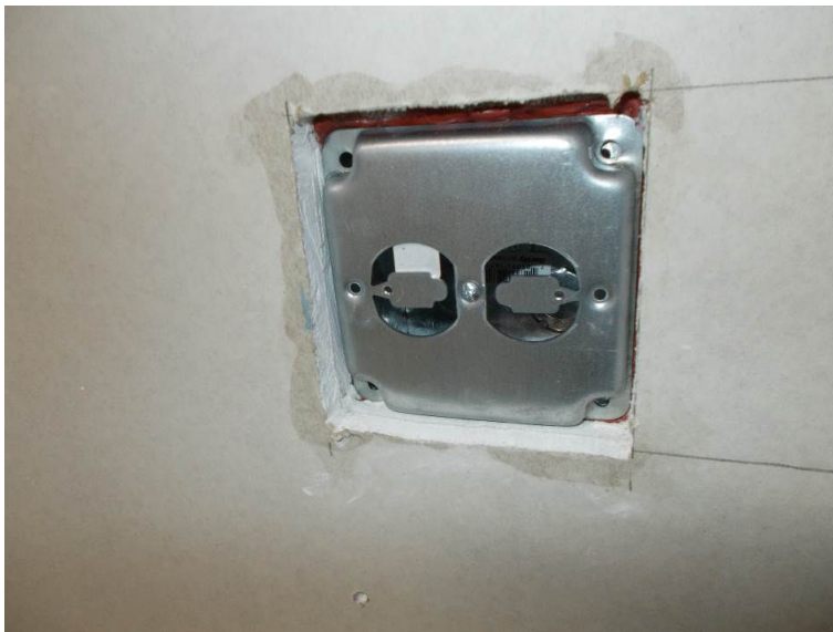
Fig. 4 Variant 4, metal box for electrical installation sealed with HILTI Putty Pad with metal cover
