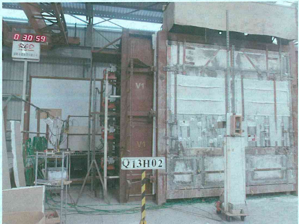
Photo 6 - The unexposed surfaces of the specimens after a heating period of 30 minutes.
