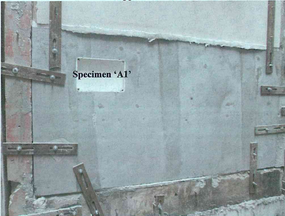
Photo 1 - The unexposed surface of the specimen 'A' before the test.
