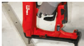
Fastening wood, e.g. Placopan®, to concrete
