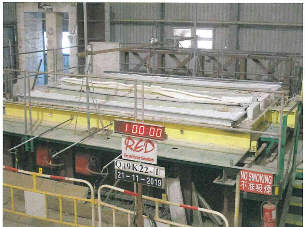
Photo 4: The unexposed face of the specimens after a heating period of 60 minutes.
