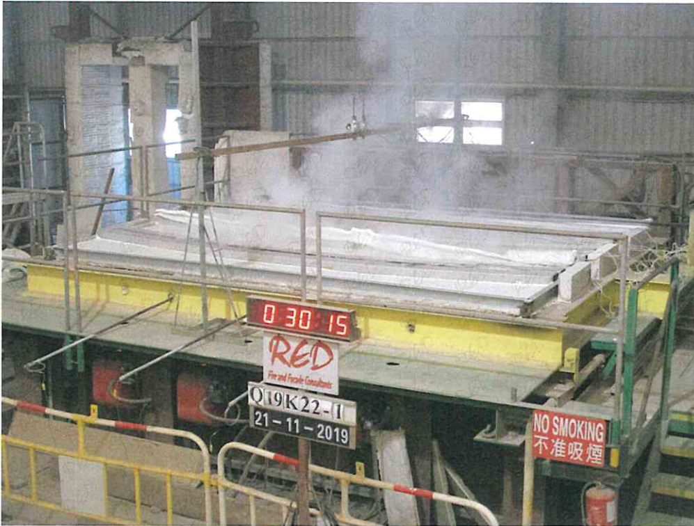
Photo 3: The unexposed face of the specimens after a heating period of 30 minutes.
