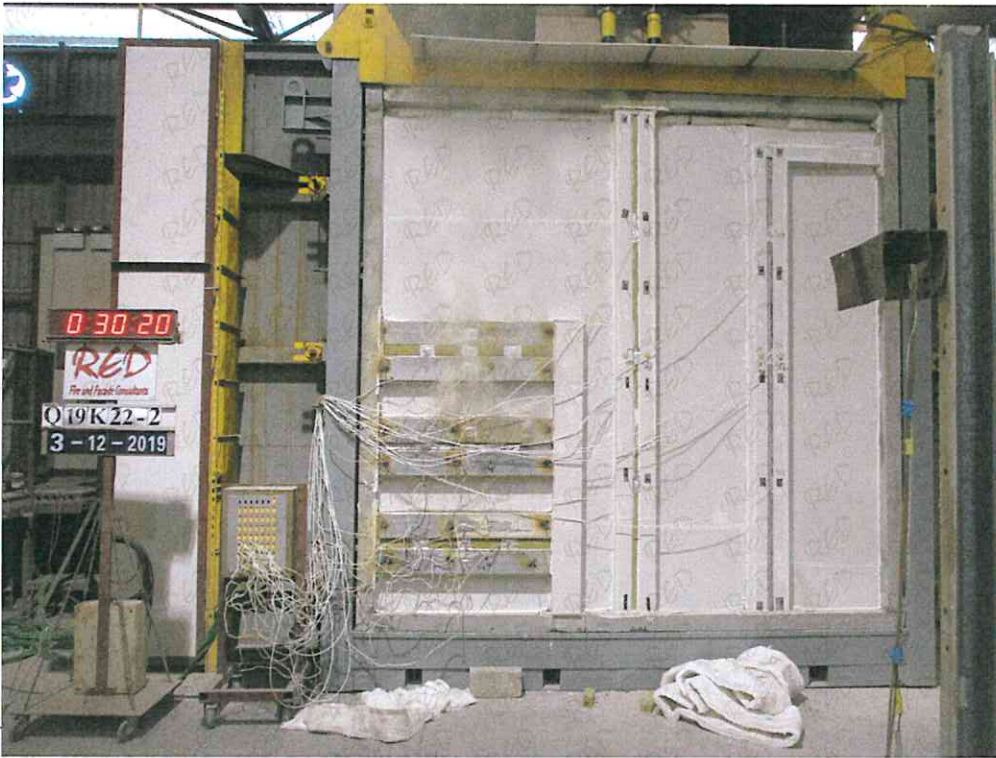
Photo 3: The unexposed face of the specimens after a heating period of 30 minutes.
