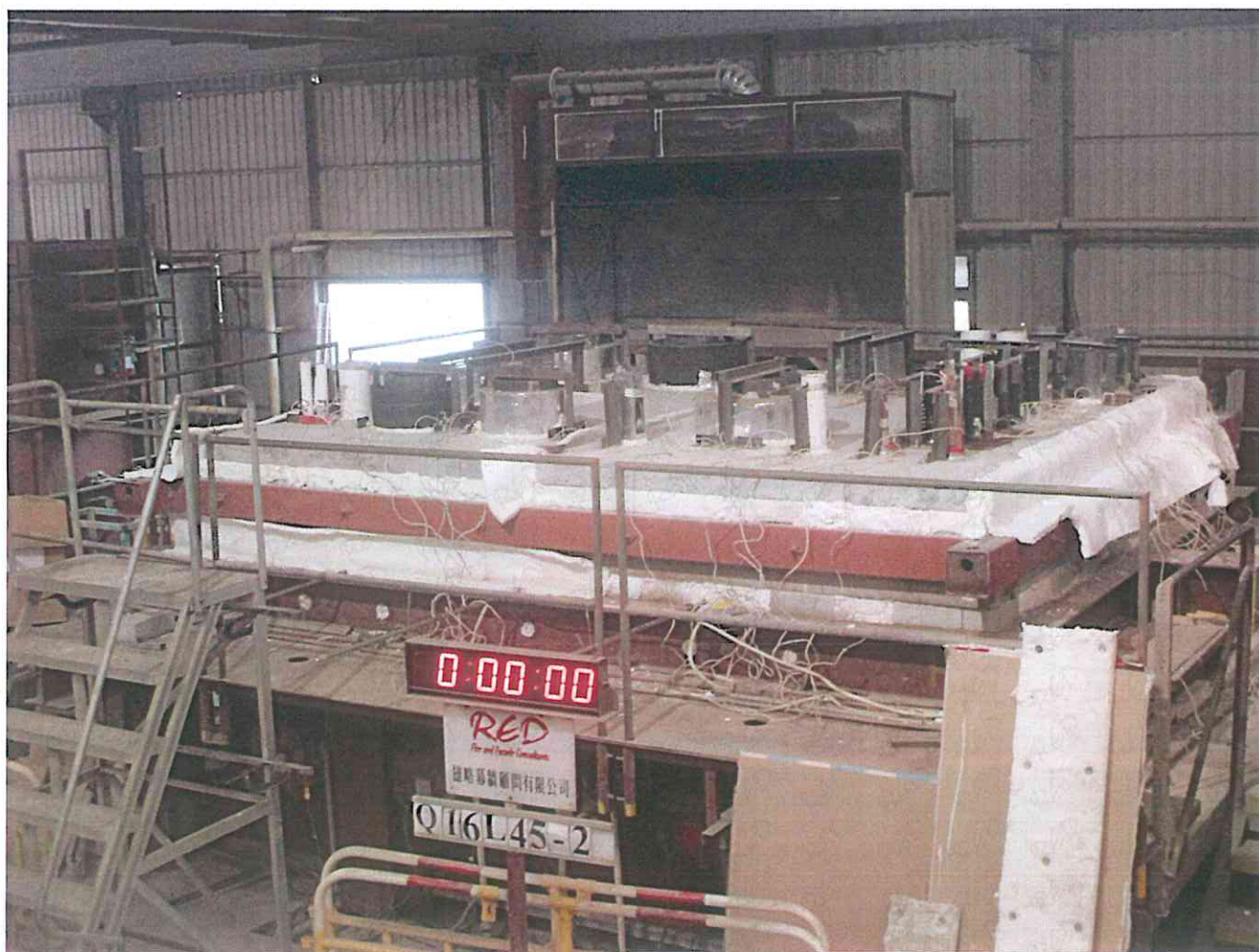
Photo 1: The unexposed face of the specimens before the test.
