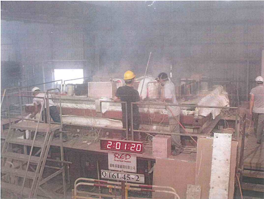
Photo 4: The unexposed face of the specimens after a heating period of 121 minutes.
