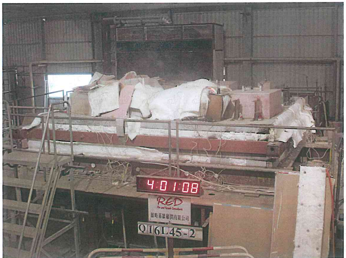
Photo 7: The unexposed face of the specimens after the test.
