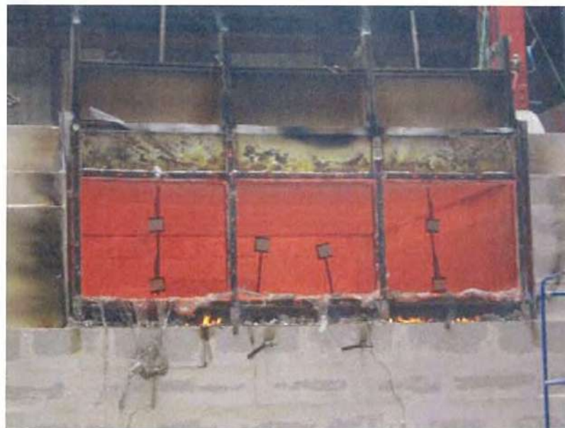
Picture C (Top) Cotton pad test positive on the horizontal seal
