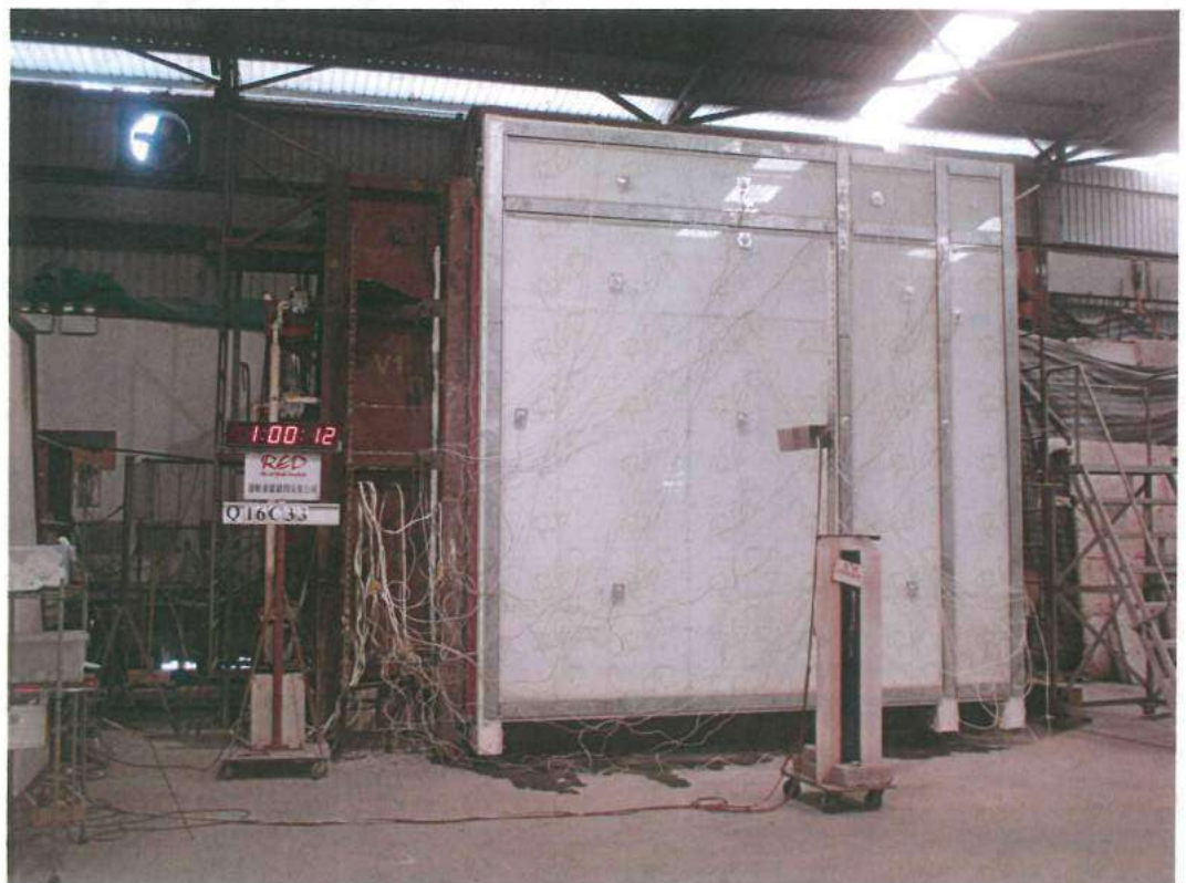
Photo 2: The unexposed face of the specimen after a heating period of 60 minutes.
