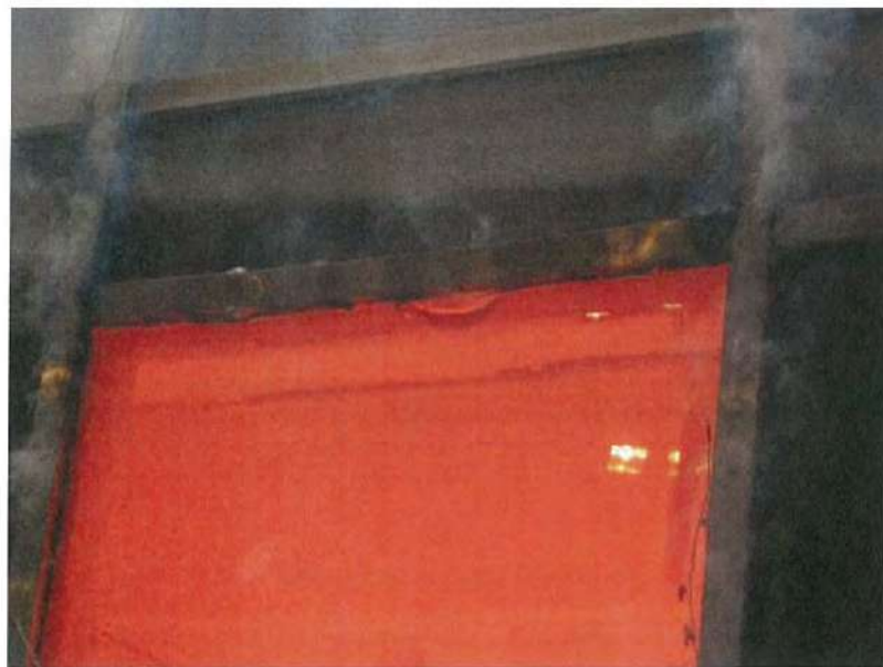
Picture A (Top) Commencement of test. Picture B (Bottom) Smelting of the glazing in the centre of the element.
