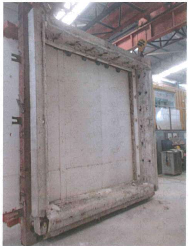
Photo 4: The exposed face of the specimen after the test.
