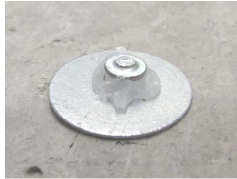
The photograph gives a visual impression of a correctly driven pin.
