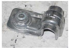
The photograph gives a visual impression of a correctly driven pin.
