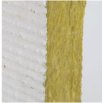
Fig. 2: Coated firestop mineral wool board [6]
